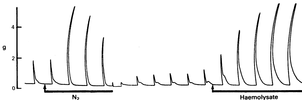
Figure 1 The effects of hypoxia and oxyhaemoglobin (haemolysate) on motor responses to field stimulation of bovine isolated retractor penis muscle. Field stimulation (10 Hz, 0.5 ms) was applied for 10 s every 3.5 min. Gassing mixture was changed from 5% \text{CO}_2 in \text{O}_2 to 5% \text{CO}_2 in \text{N}_2 as indicated at the first horizontal bar; this caused a marked but waning augmentation of the contractions. After oxygenation was resumed, the contractions were reduced in size, but were augmented again in the presence of haemolysate (oxyhaemoglobin content, 10 \mu\text{M} ).
